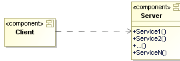
Fig. 9.3: The client-server style consists of multiple clients which request services from the central server component.
